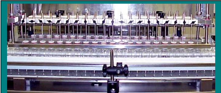
DUAL LANE CONVEYOR CONFIGURATION Shown above, nozzle centering cones provide stability to Organon's tall, skinny glass & plastic vials.
