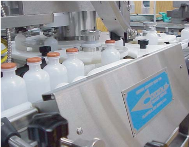
Stoppered containers are positioned to accept an aluminum cap from the feed chute.
