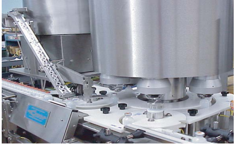
Filled and stoppered containers enter the CM200, stripping off an aluminium crimp cap from the feed chute.
