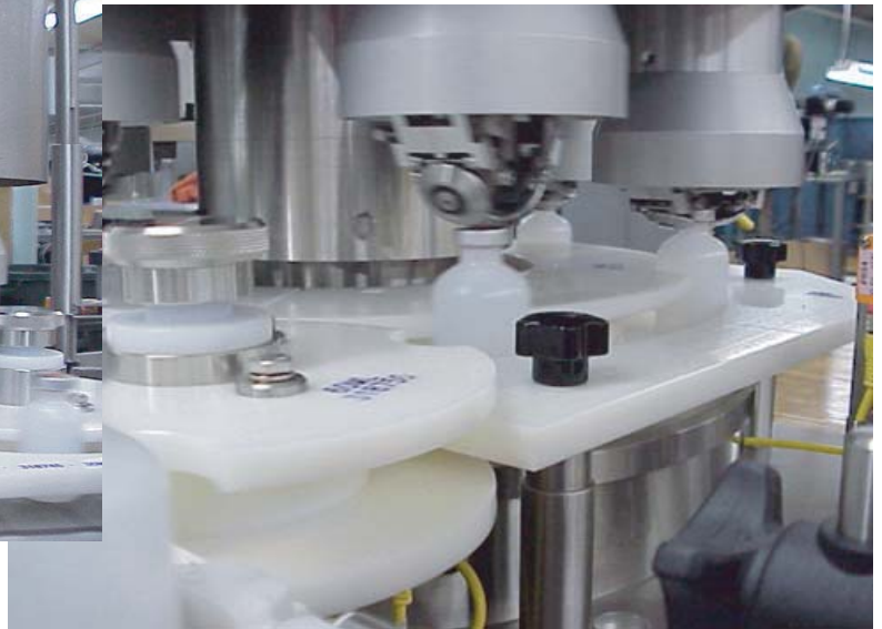
Filled, stoppered and crimp sealed containers exit the packaging line.
