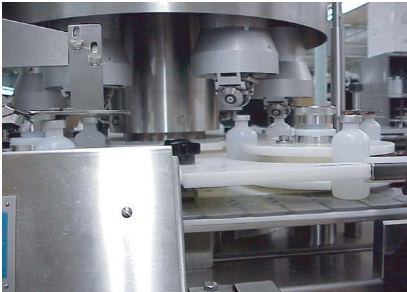
Filled, stoppered and crimp sealed containers exit the packaging line.
