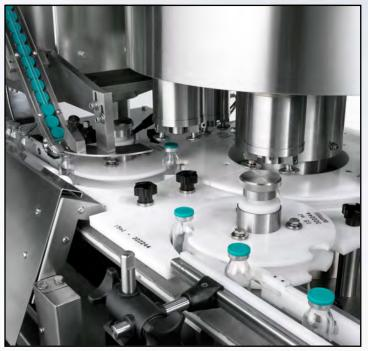
The CM200 and CM400 each have a stainless steel exterior and is equipped with a vibratory bowl, conveyor, three star-wheels and a keypad entry message center. Both accommodate tear and flip-off closures as well as line seals ranging from 13 mm - 32 mm, and handle container sizes from 2 ml - 500 ml.
