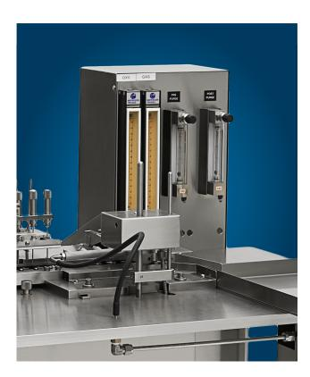
Since the blending of proper amounts of oxygen and gas is important for effective sealing of the ampule, this machine can be optionally equipped with a dual flow meter assembly that will visually indicate the oxygen and gas flow separately.
