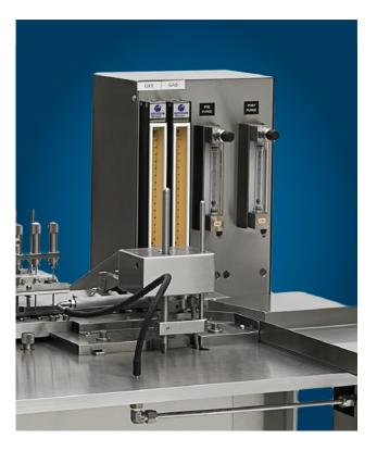
Since the blending of proper amounts of oxygen and gas is important for effective sealing of the ampoule, this machine can be optionally equipped with a dual flow meter assembly that will visually indicate the oxygen and gas flow separately.
