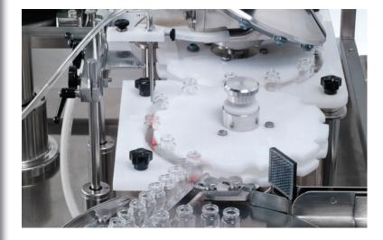
To properly align vials for filling and stoppering, each machine is equipped with a main starwheel for each container size.
