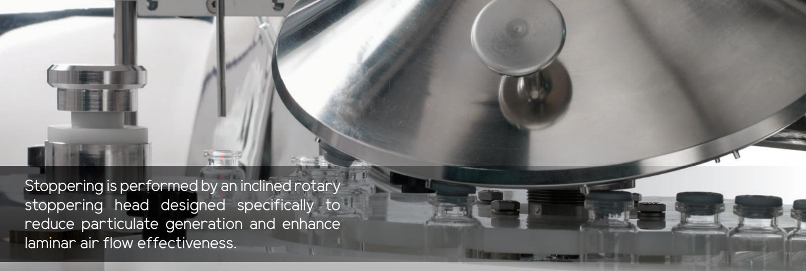
Stoppering is performed by an inclined rotary stoppering head designed specifically to reduce particulate generation and enhance laminar air flow effectiveness.
