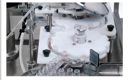
To properly align vials for filling and stoppering, each machine is equipped with a main starwheel for each container size.
