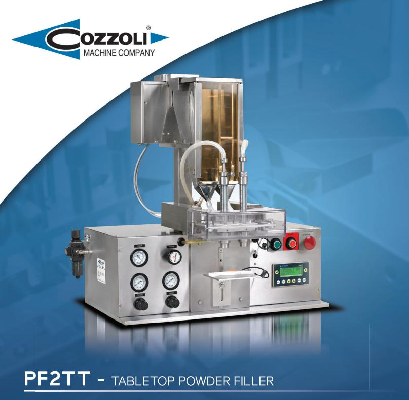
Cozzoli's PF2 Table Top Powder Filler is designed to promote the highest level of performance for both accuracy and repeatability. This precision powder filler will fill 50mg to 75grams of powder in a single dose, with an accuracy of up to +\- 1% of fill volume, depending on powder characteristics. Output speeds of 30 containers per minute can be achieved based upon operator dexterity. The compact size is designed for clean rooms, and is ideal for a lab or small production facility.
