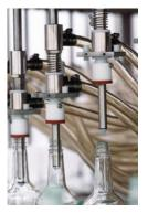
is shut down. All product overflow is drawn back to the manifold and through a trap jar, returned to the tank for re-use.
