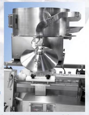
less steel exterior. All stopper contact parts are of 316 stainless steel and remove easily for sterilizing/autoclaving. The star-wheel and feed screw are constructed of durable Delrin.
