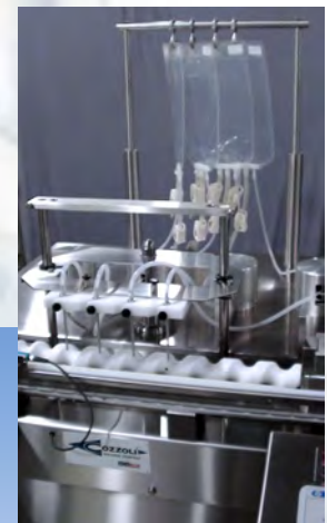
Single Use Filling Path with Plastic Bags
