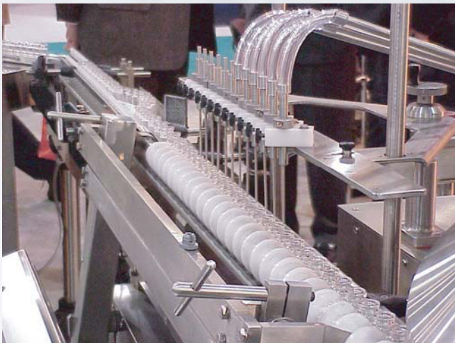
VR2/S Monoblock filler/stopper system shown.
