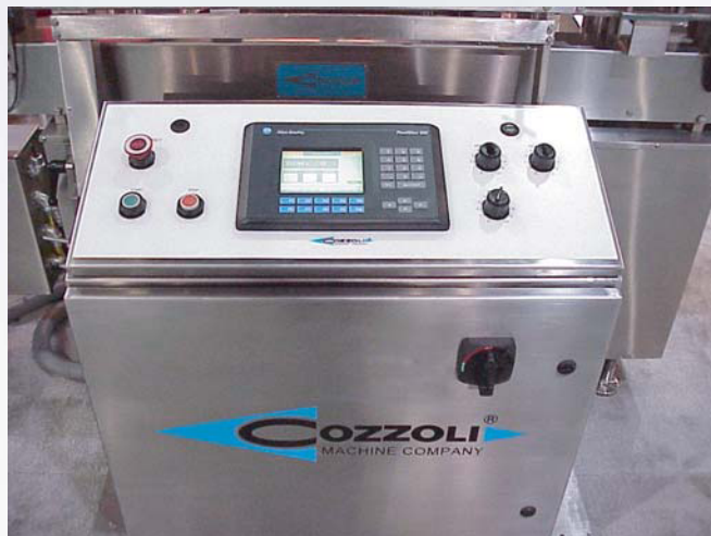
Control panel shown with optional remote umbilical mount
